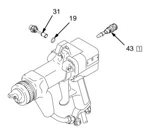
1 Apply PTFE paste to the valve housing threads (43d); Torque to 10–12 in-lb (1.1–1.4 N•m)
